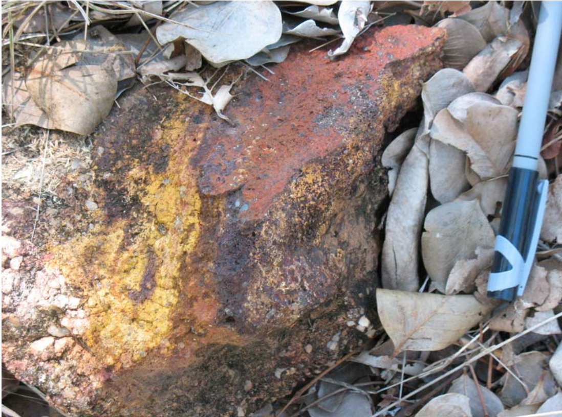
Photo 4. Riesling Prospect – High grade lead gossan containing yellow plumbojarosite ( PbFe_6(SO_4)_4(OH)_{12} ) and currusite ( PbCO_3 ) after massive sulphides – 211,177E; 7,972,633N.
