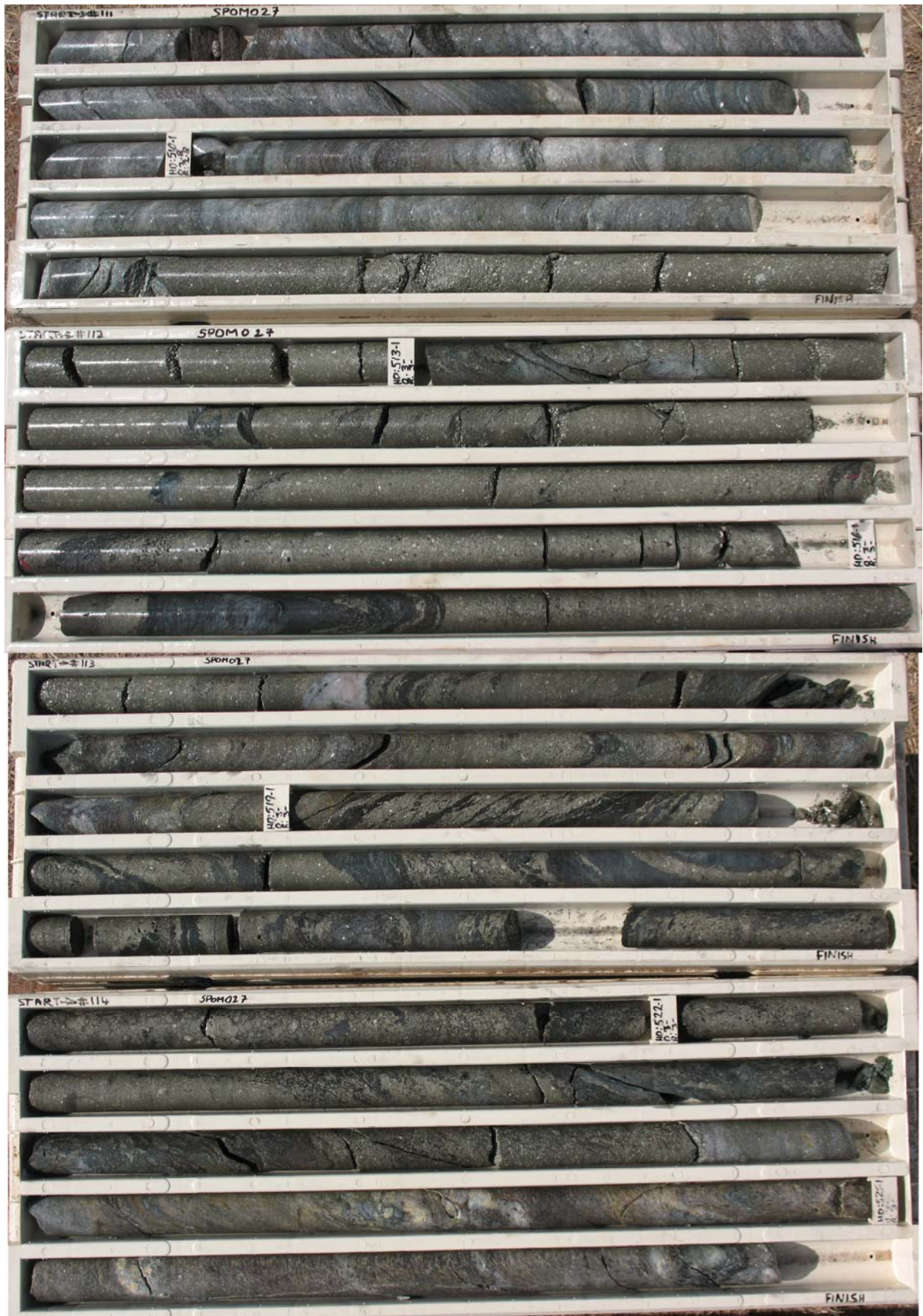
Photograph 1. Massive and semi-massive sulphide intersection between 511.7m and 524.0m in drill hole SPOM027 at One Mile. NQ core diameter is 47.6mm and length of a tray is 1 metre.
