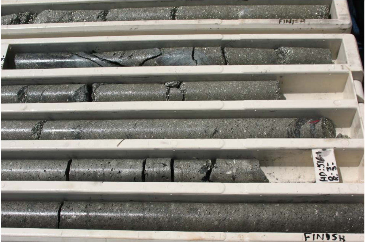
Photograph 2. Close-up photograph of massive sulphides between 533.0m and 516m in drill hole SPOM027 at One Mile. NQ core diameter is 47.6mm and length of a tray is 1 metre.
