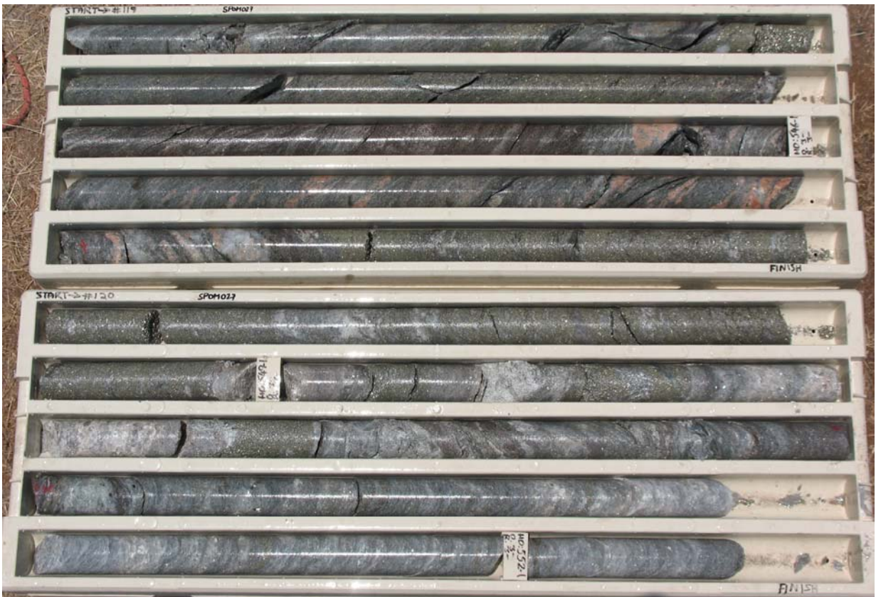
Photograph 3. Semi-massive sulphide intersections between 543.0m and 550.1m in drill hole SPOM027 at One Mile. NQ core diameter is 47.6mm and length of a tray is 1 metre.
