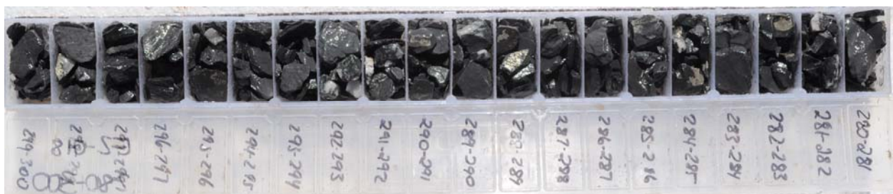
Photograph 1. Drill chips from hole EZ018 between 280 and 300m showing sulphides (pyrite) and quartz-dolomite veining in weakly graphitic dolomitic siltstones.
