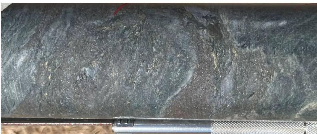
Figure 18. Core from BTDD011 (225.5m). Example of the two major types of hydrothermal alteration at Bottletree. Core sample consists of a moderately foliated meta-andesite with strong brown biotite (potassic) and later dark green actinolite (calcic) stages of alteration. Brassy yellow chalcopyrite is preferentially associated with biotite in this zone of "calcic-potassic" alteration. Alteration is preferentially focussed along pre-existing foliations.
